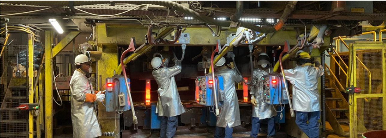
Continuous casting at Ugine melting shop
