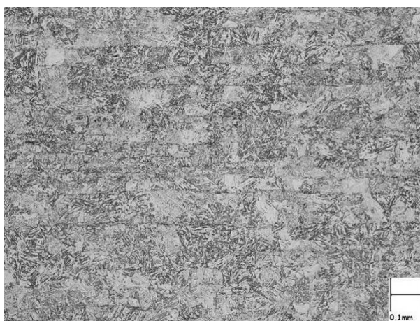
Microstructure of UGI® 4057 AIR in quench and tempered condition, observed under light microscope
