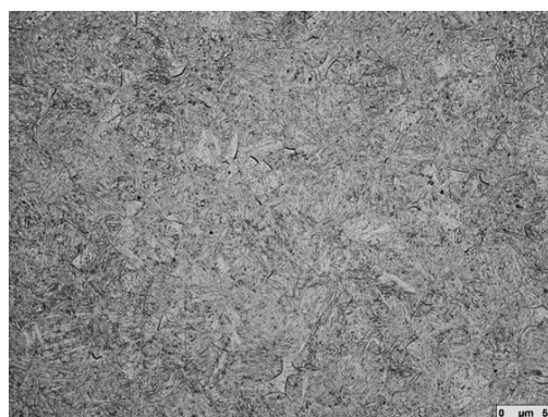
Microstructure of UGIDRILL 13 in +QT condition
