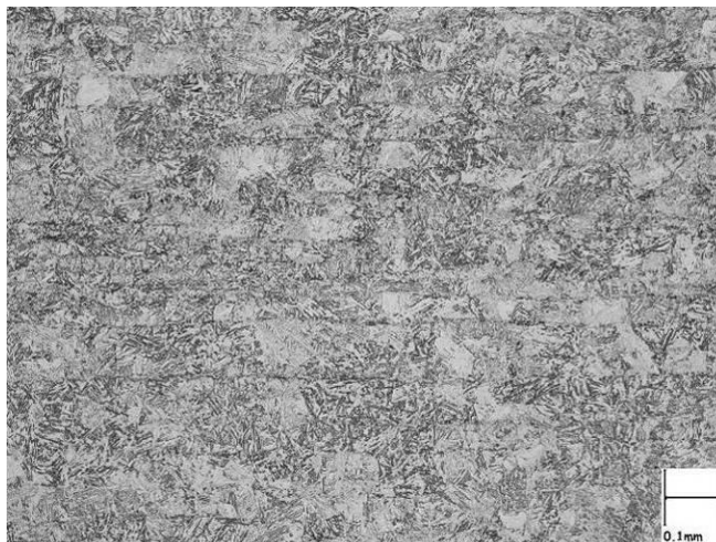
Microstructure of UGI®4057 AIR in quench and tempered condition, observed under light microscope
