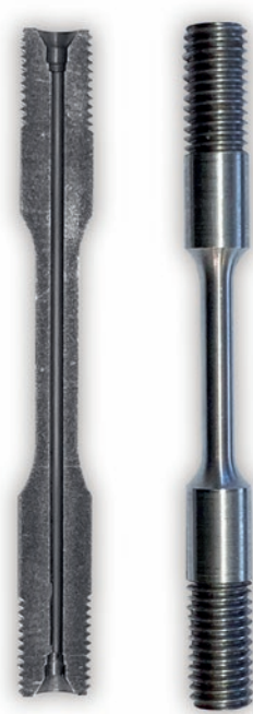
Fig. 4 - Hollow specimen for SSRT tests
