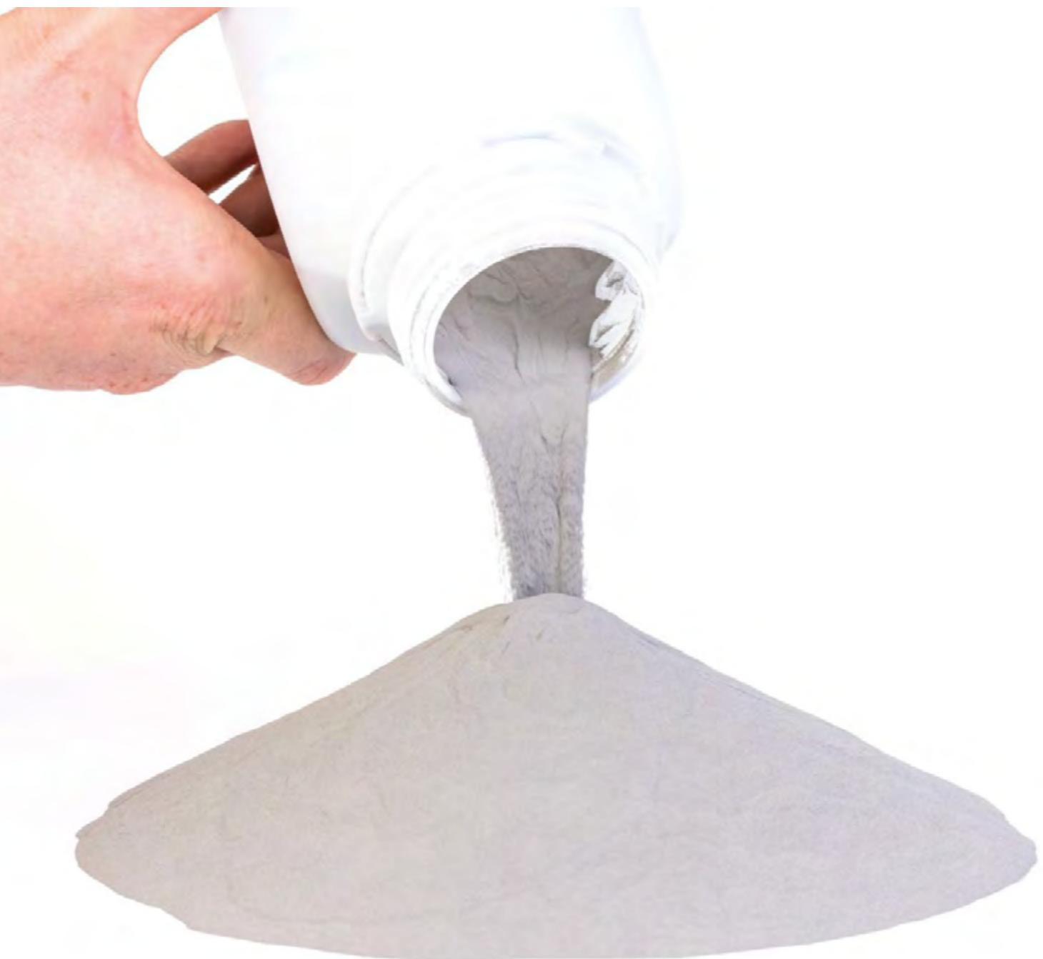
Deutsche Edelstahlwerke offers a wide range of gas atomized Fe-, Ni- and Co-based metal powders. These are ideally adapted for additive manufacturing.
