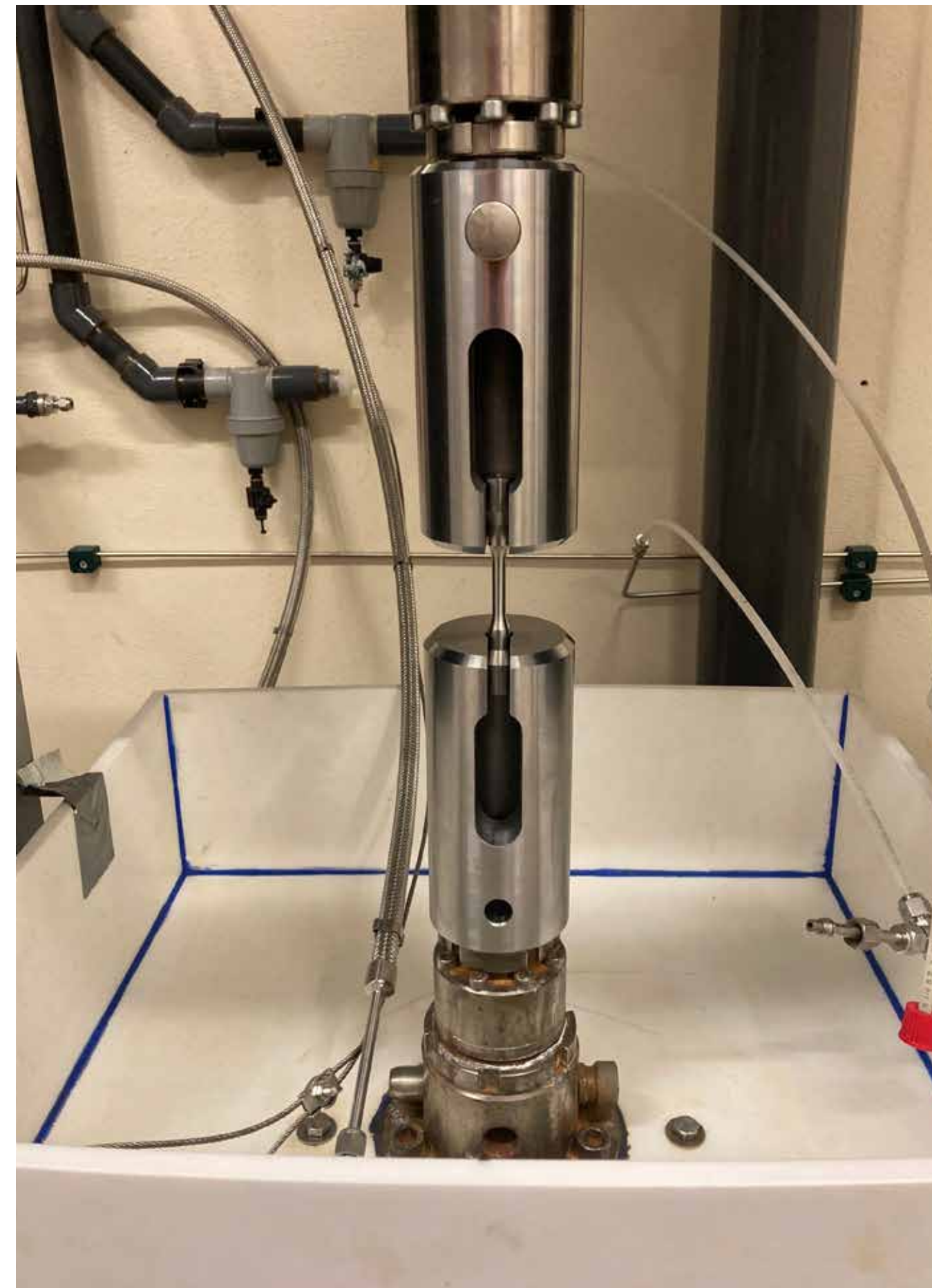
Hydrogen Laboratory: Slow-speed traction
