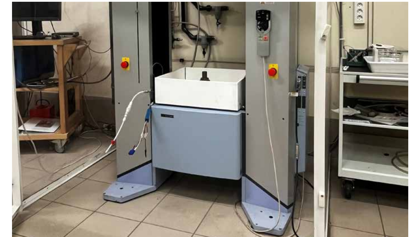
Hydrogen Lab: slow-speed tensile testing
