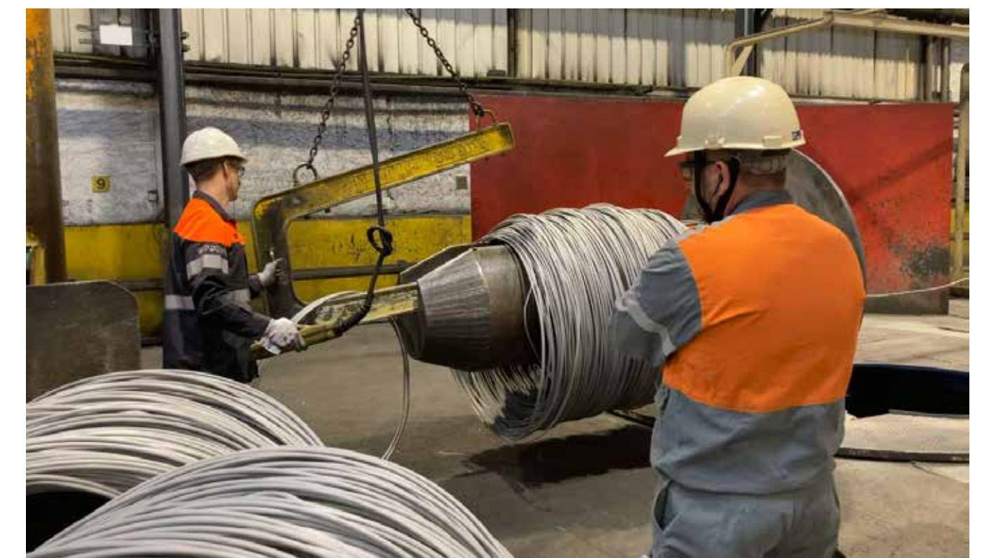
GESiM 2025-2026: wire coil unwinding area - drawing shop in Ugine
