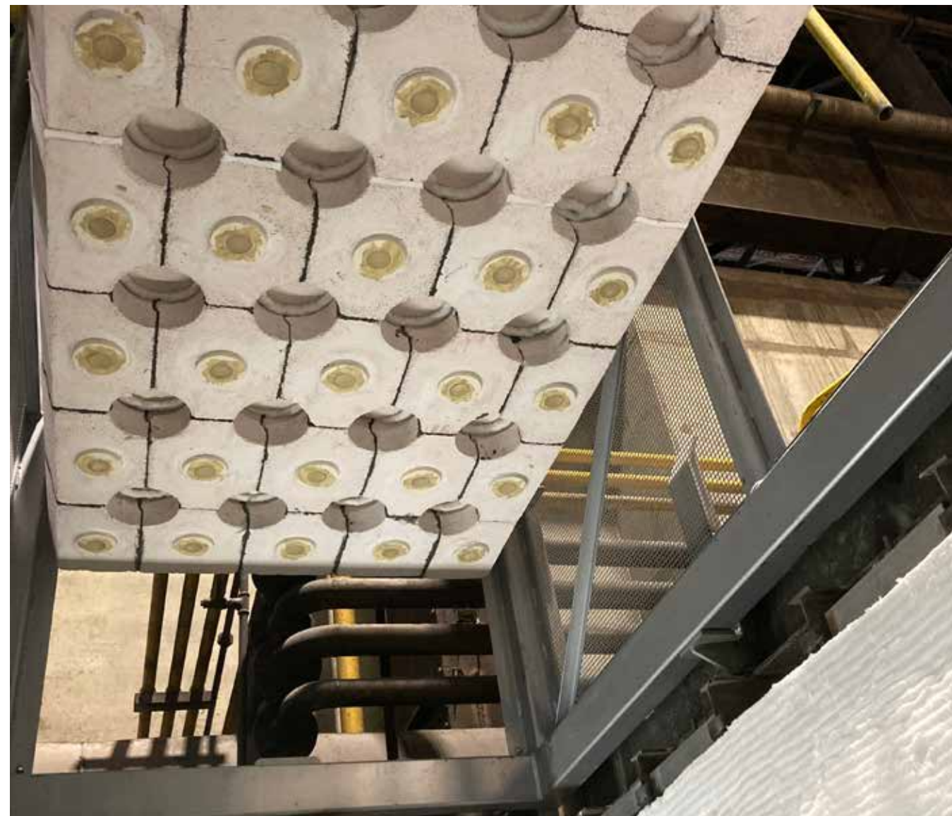
New roof in Zone 1 of the reheating furnace before the rolling mill
