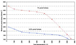
The temperature-stress-time relationships that are important for **Ferrotherm® 4828** from a creep point of view are presented in the graph below:
