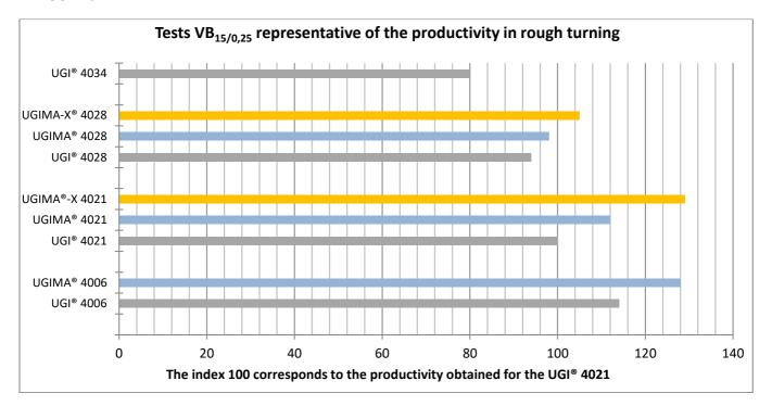
The application of the UGIMA®-X process to grade 1.4021 also ensures excellent reproducibility of machinability from one heatto the next, and therefore from one material batch to the next, a dispersion that is stronger with UGI® 4021 and UGIMA® 4021.
