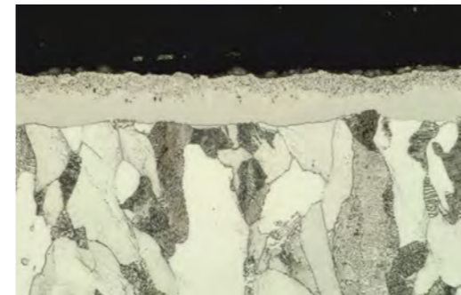
ETG® 25, 520 °C 10h, K_N = 2 , Nital etchant
